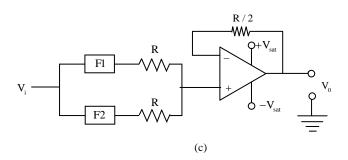
The cut-off frequencies of F1 and F2 are  $f_1$  and  $f_2$  respectively. If  $f_1 < f_2$ , the resultant circuit exhibits the characteristics of a
