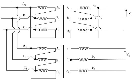
The phase different (in degree) between voltage  $V_1$  and  $V_2$  is \_\_\_\_\_\_.
