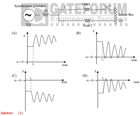
**Exp:** For generator  $\delta$  is +Ve. After fault  $\delta \uparrow$  increases
