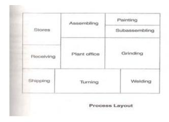
Figure 6.1: A Sample Process Layout
