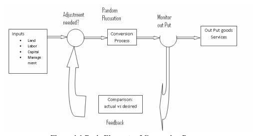
**Figure 1.1 Basic Elements of Conversion Process**
