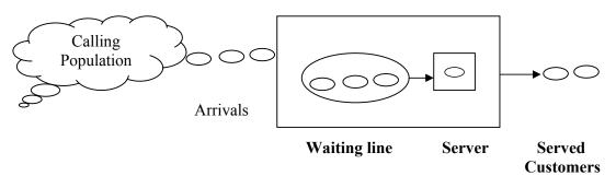
Fig. 4.3Basic Structure of a Queuing System
