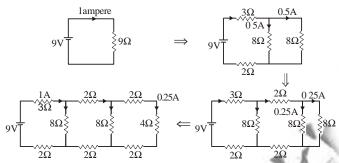
The current divides into two equal parts if passes through two equal resistances in parallel.
