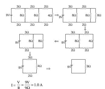
The flow of current in the circuit is as follows.
