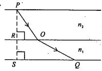
What is the optical path of light ray traversing the path POQ across two media of refractive indices  $n_2 = \frac{3}{2}$  and  $n_1 = \frac{4}{3}$  (PR = a, RS = b, RO = x, SQ = y)?
