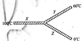
Three rods X, Y, Z of same dimension having thermal conductivities 3K, 2K, K respectively are arranged as shown in the above figure. Their ends are at  $100^{\circ}$ C,  $60^{\circ}$ C and  $0^{\circ}$ C respectively. What is the temperature of the junction?
