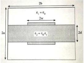
Where a =b=2.5cm, d=0.5,  $\omega$ =1cm,  $\varepsilon_1 = \varepsilon_0$ ,  $\varepsilon_2 = 2.35\varepsilon_0$ and the thickness of the strip is neglected. The potential difference applied between the outer metal shield and the inner strips is V<sub>d</sub> =100mV.
