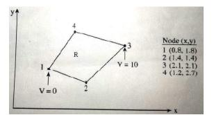
12. Solve La Place equation inside the region R as shown in the figure by Finite Element Method (FEM).
