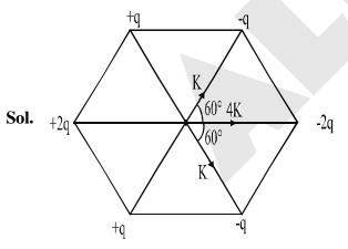
Resultant is 6 K along OD. For every point of POR there are two charges of opposite sign and equal magnitude at equal distance.
