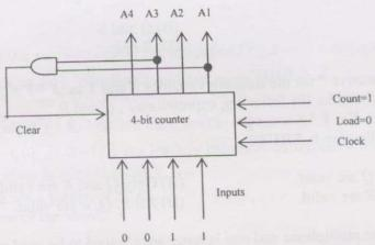
Assume that the counter and gate delays are negligible. If the counter starts at 0, then it cycles through the following sequence:
