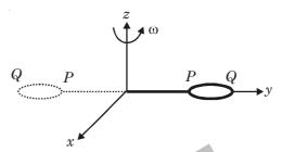
Now consider two similar systems as shown in the figure: Case (a) the disc with its face vertical and parallel to x-z plane; Case (b) the disc with its face making an angle of  $45^{\circ}$  with x-y plane and its horizontal diameter parallel to x-axis. In both the cases, the disc is welded at point P, and the systems are rotated with constant angular speed  $\omega$  about the *z*-axis.
