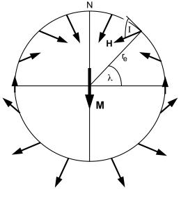
**Figure 1.3** Geocentric axial dipole model. Magnetic dipole *M* is placed at the center of the Earth and aligned with the rotation axis; the geographic latitude is  $\lambda$ ; the mean Earth radius is  $r_{e}$ ; the magnetic field directions at the Earth's surface produced by the geocentric axial dipole are schematically shown; inclination, *I*, is shown for one location; N is the north geographic pole. Redrawn after McElhinny (1973).
