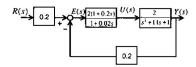
The steady state gain of the closed loop system, between output Y(s) and set point R(s), is
