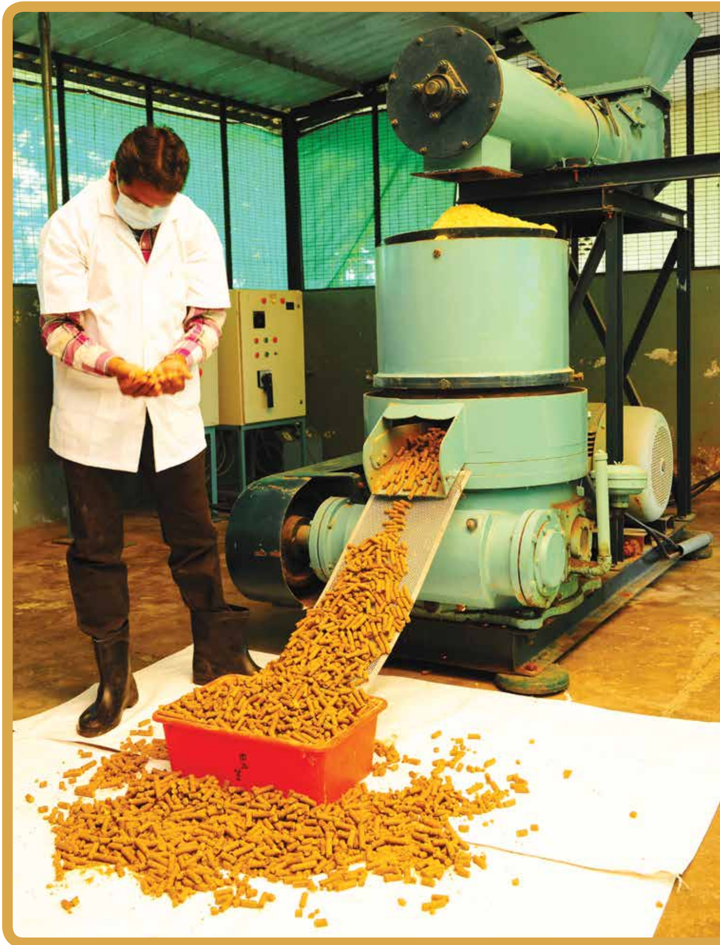
Production of straw based feed pellets on a pilot scale
