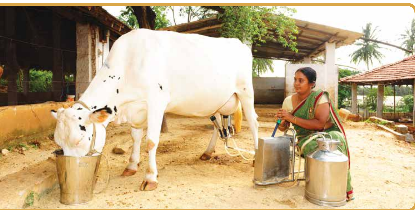
Indigenously developed hand-held milking machine in operation
