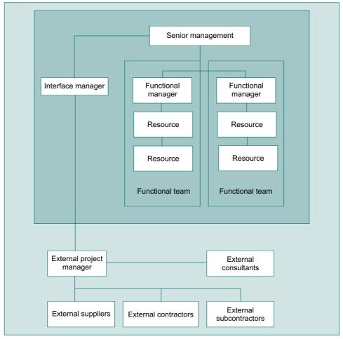
Figure 1.10 Typical external project management arrangement
